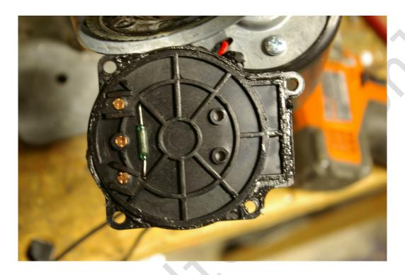
Simply remove the old reed switch and replace it with a new unit.
