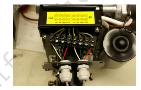
On the Mini-RAS Rotator, remove cover from the Rotator and pull out the 8 pin terminal strip. The Elevation connections are on the Right of the above picture and the Azimuth is on the Left. Pin 1 of the Elevation motor is on the right and pin 4 of the Azimuth Motor is on the left.
