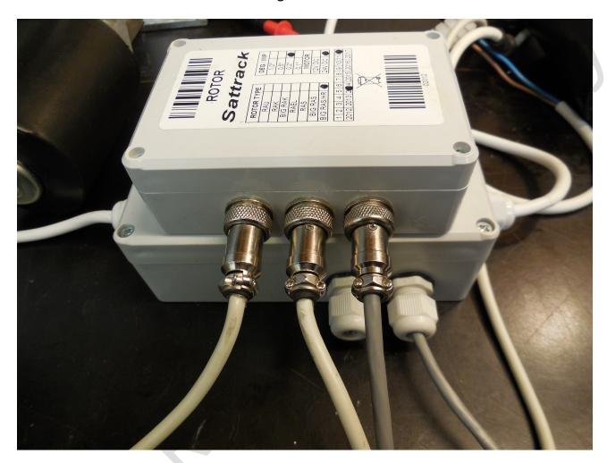
When installing any rotator, care must be taken to ensure that the antenna and rotator cables are installed, so that it is not damaged while the antenna is rotated through it's normal azimuth operating angular travel. When installing an Alfa Rotator, that normal azimuth operating angular travel can be up to 720 degrees.
