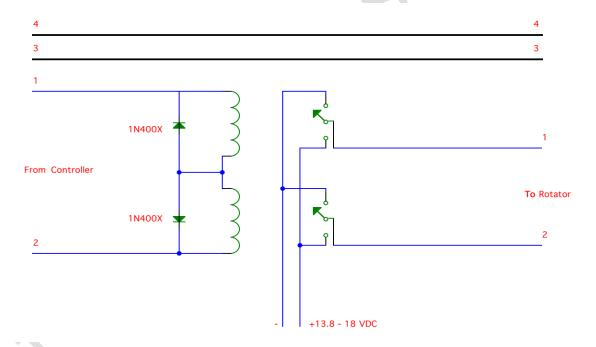
Relays chosen should be suitable for the proper coil voltage, as well as appropriate current carrying capacity of the contacts. A relay capable of 5 to 10 amps DC is adequate. The diodes are general-purpose 1 amp style such as the 1N400X series.
